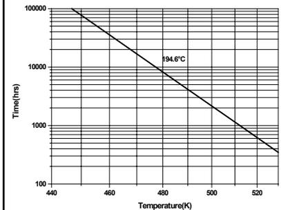
Thermal Endurance characterisation has been assessed on the resin base using twisted pair ageing according to the procedures called up in UL1446.
